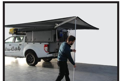
**Step 8 :** With the foot of the centre support leg on the ground, raise the awning slightly, and tighten thumb screw on the pole.
