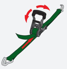
**4.** When lashing is tight enough, put handle in the most downward position to lock it and prevent breaking.
