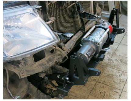
21. Mount the winch (not supplied) following the winch installation instructions supplied with the winch manufacturers.
