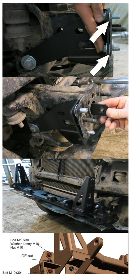
17. Place bolts M10x30 (B) with washers penny M10 (M). Push support bracket to the front of the chassis. If there is a gap of more than 2mm, place washers penny M10 (M) inside.
