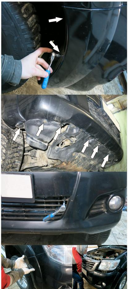
4. Remove lower bumper retaining screws and scrivets.
