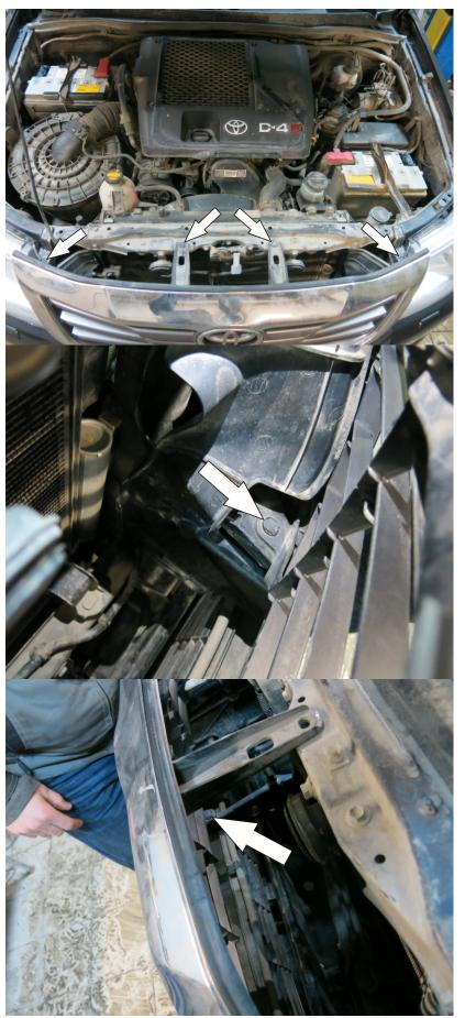
1. Open the bonnet and remove all scrivets holding the grill in place.
