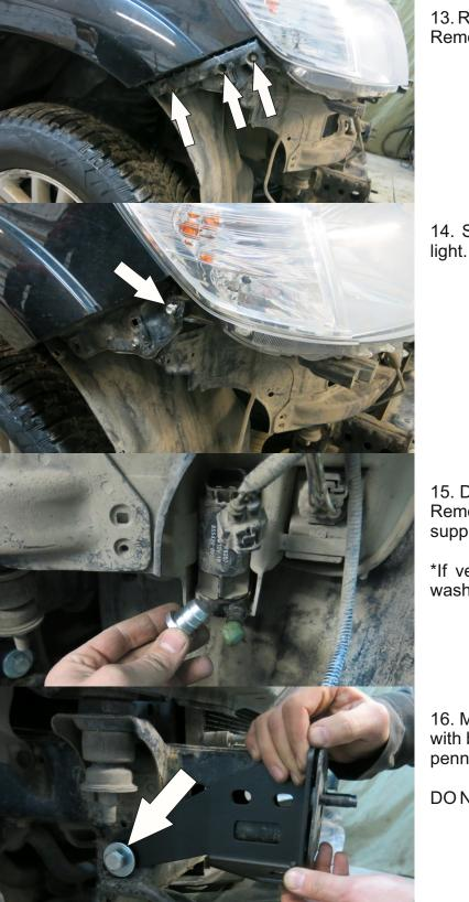
13. Remove M6 bolts and scrivets. Remove plastic side fittings.
