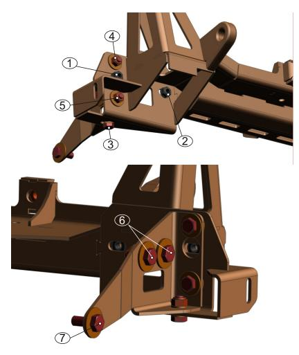
20. Align winch bracket (2) horizontally and vertically.
