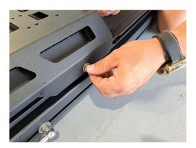
Once all the bolts are in place, you can fasten all the bolts down completely with a 5mm allen key.
