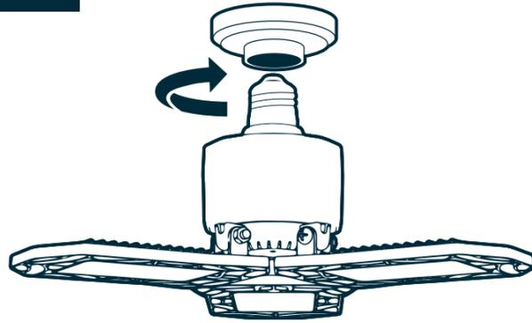
Simply screw the High Bright 6000 into any any standard (E26), non-recessed light bulb socket.
