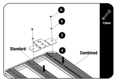
Flip the Rack so that the bottom of the Rack faces up. Insert two M8 x 16 Hex Bolts (Item 4) into the Combined slat and Standard slats machined slots as shown.
