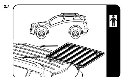
With the help of a friend, flip the rack over, right side up and place it onto the rails of the vehicle
