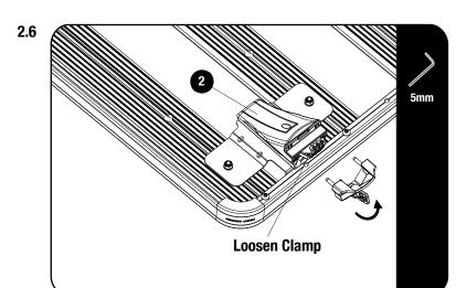
Unlock the covers on all four Feet and loosen the clamps using a 5mm Allen Key.
