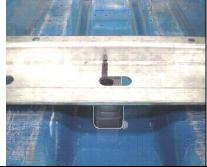
**2.14/-** Bolt frame down through drilled holes using four (4) M10x40mm bolts, M10x70x40 flat plates inside the vehicle at the front.
